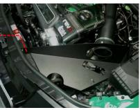
Undo the nut on the red power terminal located on the suspension turret and fit the rear heat shield bracket onto the stud and refit the nut. Place the middle heat shield bracket onto the original airbox mounting and secure using the OE bolt. Leave all brackets slightly loose to allow for adjustment.
