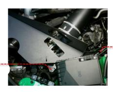
8 Install the Revo intake joiner hose and hose clamps.
