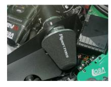
Adjust the heat shield brackets and intake joiner hose to ensure sufficient clearance around the intake system. Tighten all hose clamps and bracket fixings.
